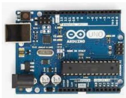
**Gambar 2.1 Board Arduino Uno**
