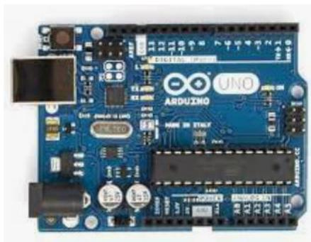
**Gambar 2.1 Board Arduino Uno**
