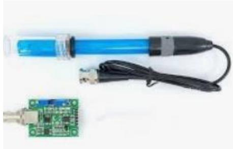
**Gambar 2.2 Sensor PH4502C**
