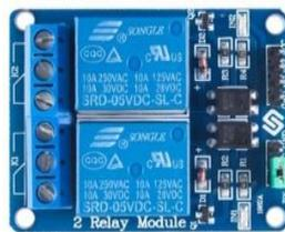
Gambar 3. Modul relay 2 saluran 5v
