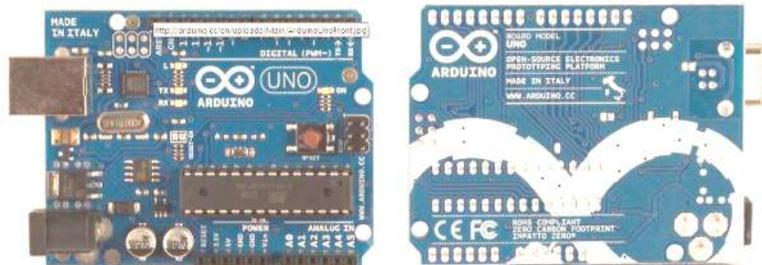
Gambar 2 Arduino Board
